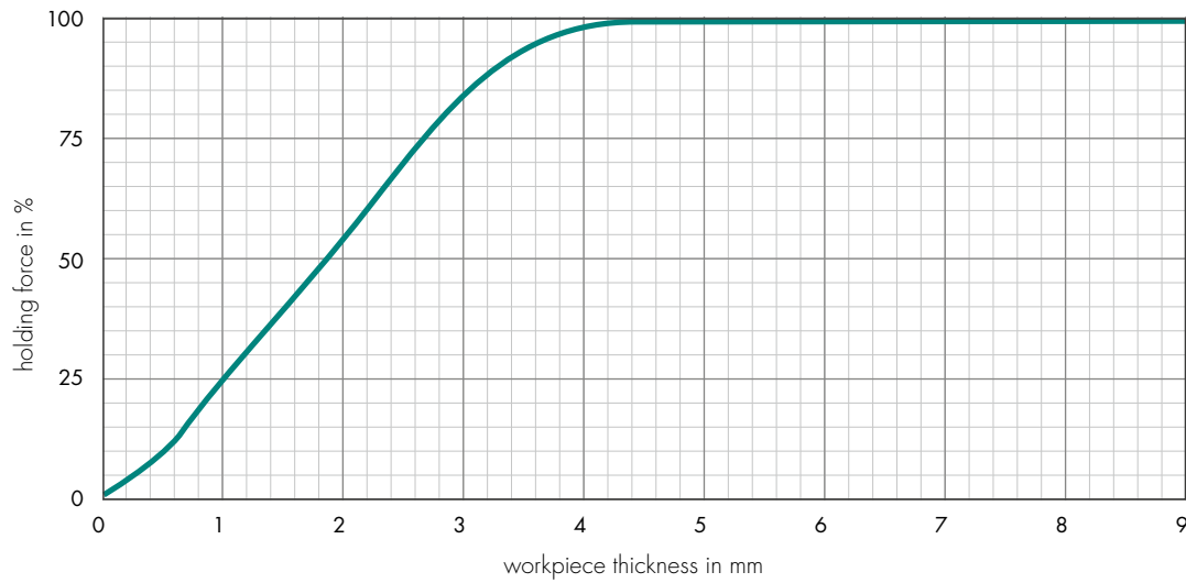
SAV 244.01 transverse pole pitch 1.9 mm
