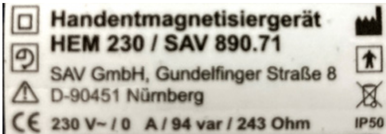
Fig. 4: Type plate SAV 890.71
