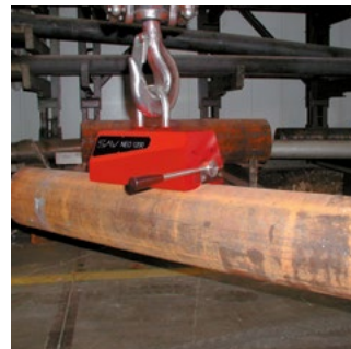
Modell 1200: Massives Rundmaterial
